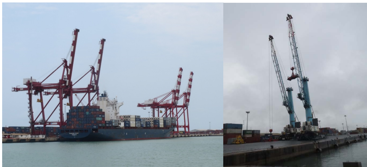
Figure 17: Picture of Four Ship-to-Shore Gantry Cranes at Benin Terminal (left) and Two of APMT's MHC (right), September 2015
